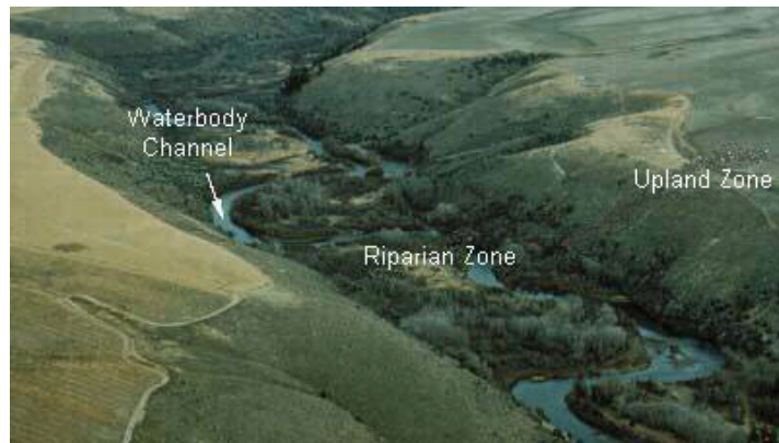
Figure 13: The waterbody channel, riparian zone, and upland zone are three zones referred to when discussing watershed management.
