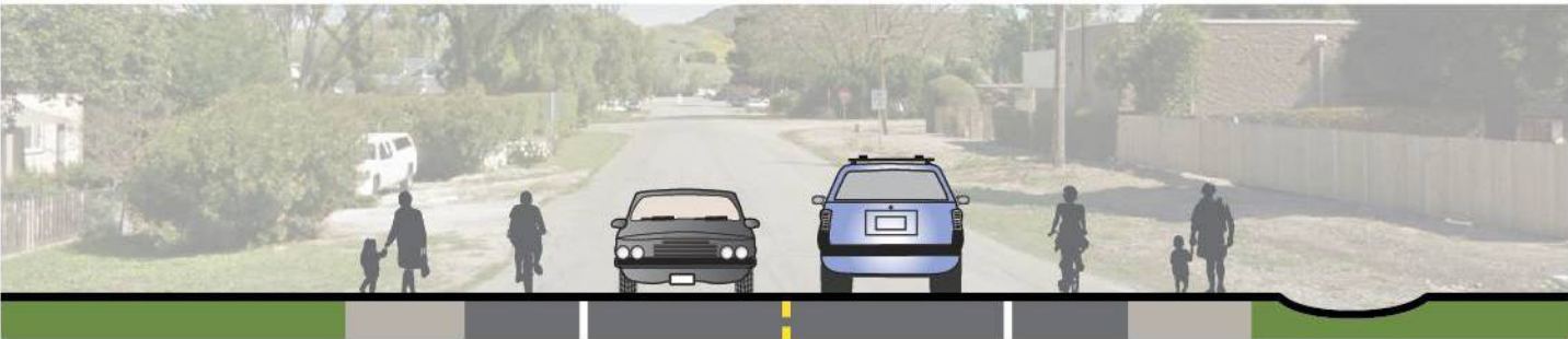
Walking paths and striped bike lanes on both sides of the street
