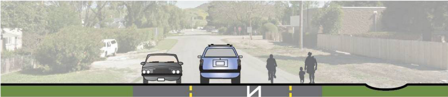
Shared pedestrian and bicyclist path on one side of the street
